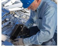
X-ray guns have been especially slow at measuring Mg, often taking up to a minute to measure 0.5% Mg in a 6063.
