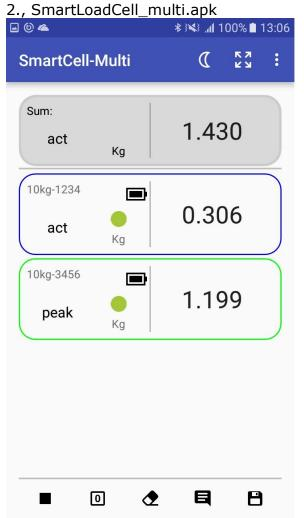
This application can be connected to maximum 7 SmartLoadCell modules (load cells). All load cells actual and maximum values can be monitored on the same screen. Graphs of the measurements can be viewed in the history.
