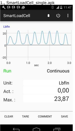
This application can connect to 1 SmartLoadCell module (1 or 2 channel ones too). Measurement graph is displayed real time and in the history too. SmartLoadCell\_single application has 4 different measuring modes. Relevant modes for this application:
