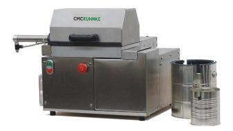
The AGS-3000 SEAM Saw is engineered to automatically cut can Double Seams precisely and efficiently, giving you a clear image for highly reliable visual inspection and analysis. This automatic saw features a rugged design that will provide you with years of quiet, trouble-free performance.
