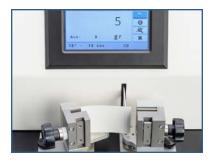
With only one button, the Crease and Board Stiffness tester is very easy to use. The zero button is used to zero the instrument before each test.
