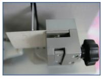
The sample is clamped with a strong spring loaded clamp. Opening and closing the clamp is done by turning the screw. The maximum sample thickness is 4mm.
