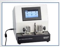
The left clamp is fixed at a 50mm distance and rotates 15 degrees. The right clamp turns 90 degrees on 10mm. For Crease line, bending resistance and spring back.
