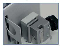
The clamps are easily interchangeable. In addition to square clamps also round cornered clamps are available according to the Philip Morris standard.
