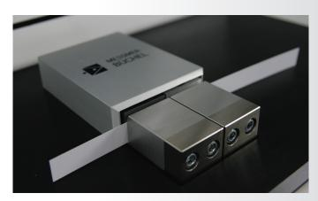
The clamps are mounted on special, low friction gliders. Long term precision and perfect parallelism are assured by a self-alignment mechanism unique to Messmer Büchel.
