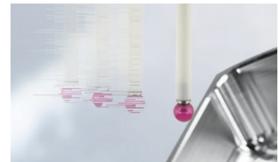
The probes moves at high speed, so that measurement times are significantly reduced.
