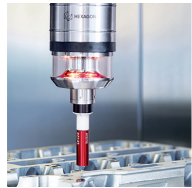
Determination of the workpiece temperature directly on the machine - thanks to the patented temperature measuring unit
