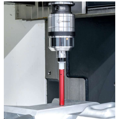
Determination of the workpiece temperature: Before, during and after machining.
