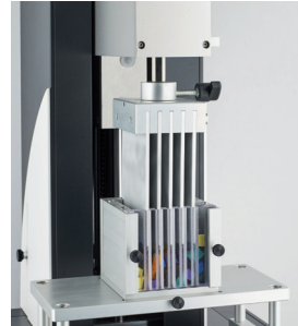
KRAMER CELL 5 BLADES ALUMINIUM+PLEXIGLASS (PN 130094) Hardness and tenderness on small samples Required table PN 310106.
