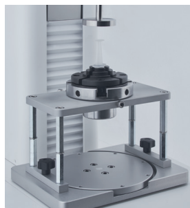
SYRINGE TEST BENCH (PN 130145) Study of needed force to use syringe.
