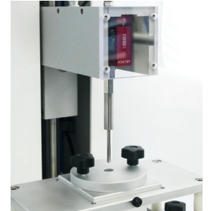
COMPRESSION CELL FOR FILM (PN 130031) Accessory to measure strength of film Required table PN 310106.
