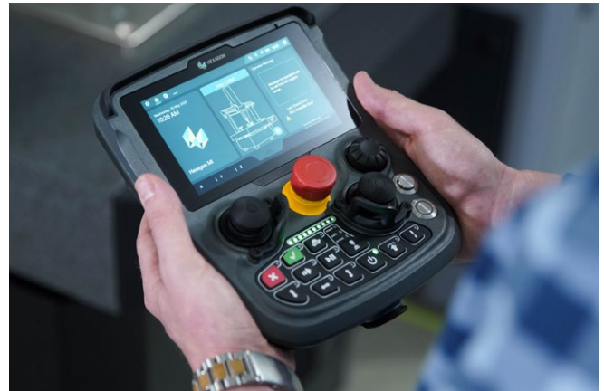
More than a jogbox, this wired or wireless handheld digital control center (dCC) enables quick access to metrology software applications from anywhere around the CMM
