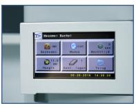
Testing is quick and easy. Parameters are software controlled and can be adapted, such as gap height, auto test mode, auto-zero and dwell time.
