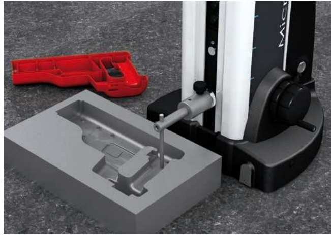
Measurement of a plastic injection mould for a drill plastic cover
