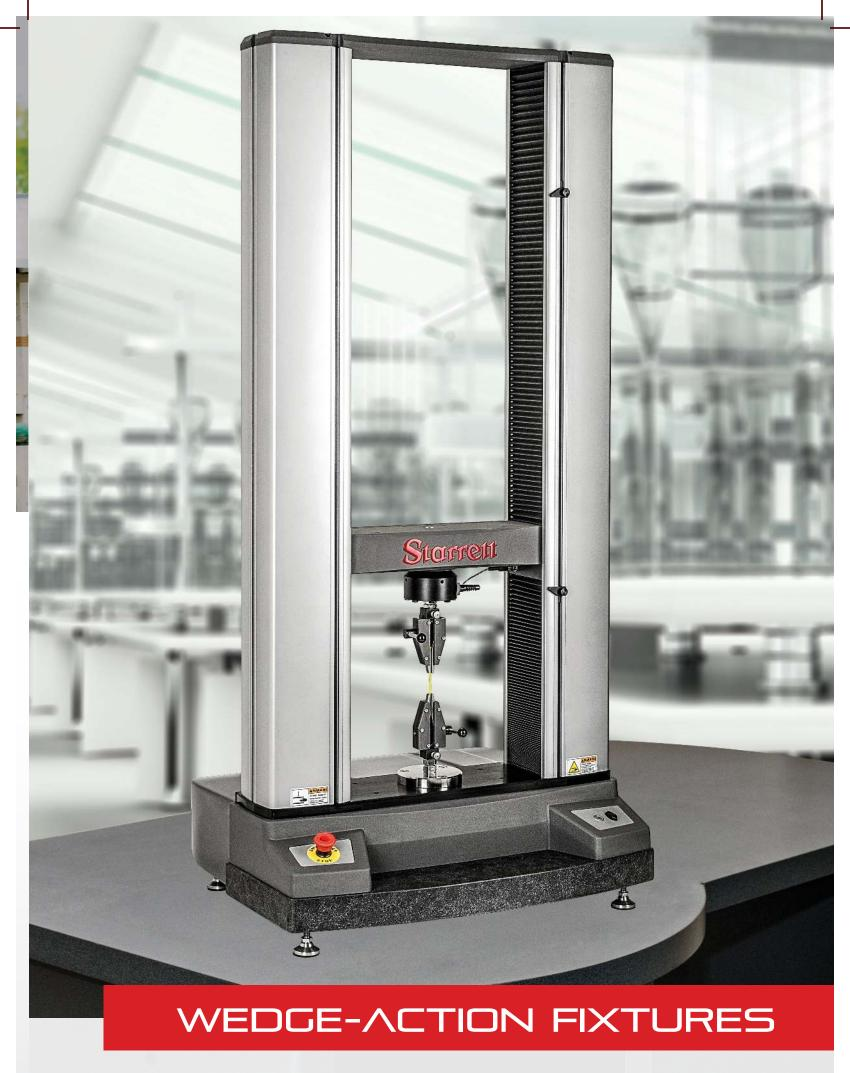
Wedge fixtures are self-tightening. Starrett offers a variety of different wedge-action fixtures with various face types for flat and round sample dimensions.
