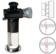
Brinell HBWT tests
