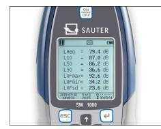
Data logging function with date and time in the device...
