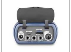
... and data transfer using MicroSD (4G) memory card (included in delivery), RS-232 or USB
