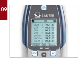
Data logging function with date and time in the device...
